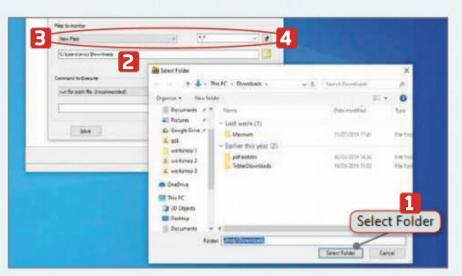
A folder selection window opens. Locate the folder you want to monitor, then click the Select Folder button. 1 It appears in the box. 🔼 We're monitoring for all types of new file, so we can leave the other options in the 'Files to monitor' section set to the defaults: New Files 3 and ".\*". 4
