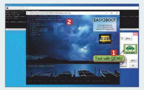
If you want to check that the software is working, click the 'Test with QEMU' button. 🚺 This launches the boot menu in a simple emulation Window 2 so you can see that it works. We found this very slow on our PC, but don't panic - the finished version will perform much better. Shut down QEMU and load your other ISOs.
