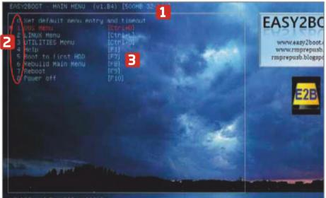
Now when you reboot your PC with the USB device connected, it takes you to the Easy2Boot menu. 11 Here you can use the arrow keys to navigate to the option you want. Alternatively, skip to the option using the number keys 🔼 or open the menu using the shortcut. 3 F8 takes you back to the main menu.
