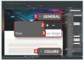
To change the typeface and text size, select the text, then go to the Panels menu and choose Style Properties. Expand the General section 💶 and click the plus button 🔼 to add a font family, then select it and set the size you want. El Expand the Colors section 4 to change an item's foreground or background colour.
