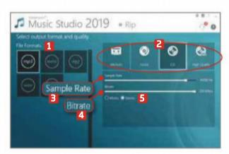
Click Next, then select a format for your ripped tracks - MP3, WMA, OGG, WAV or FLAC 1 - and the quality you require. 2 You can adjust the sample rate **3** and bitrate **4** using the sliders, and select mono or stereo. 5 Choose an output folder and naming format, then let the software get to work.
